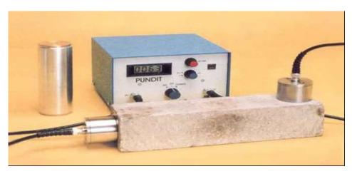
Figure 1. Pulse velocity testing equipment (PUNDIT).
