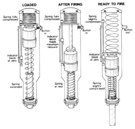
Figure 3. Operational system of a Schmidt Rebound Hammer (SRH).
