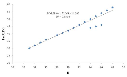
Figure 5. Rebound number/compressive strength calibration curve.
