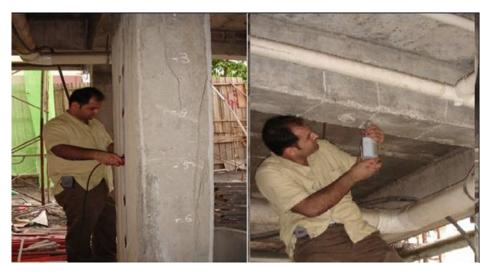
Figure 4. UPV and SRH tests in site.
