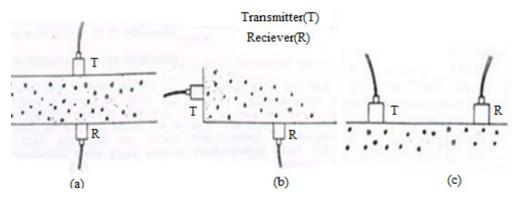
Figure 2. Direct (a), Semi-direct (b) Indirect (surface) transmission (c).
