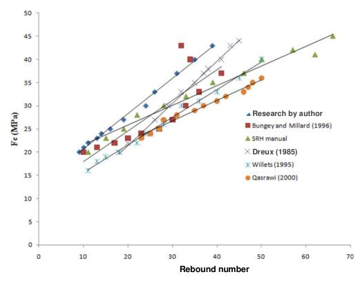
Figure 7. Comparison of Schmidt Rebound Hammer (SRH) test with others.
