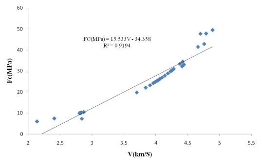
Figure 6. Ultrasonic Pulse Velocity (UPV)/compressive strength calibration curve.
