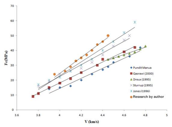
Figure 8. Comparison of Ultrasonic Pulse Velocity (UPV) test with others.
